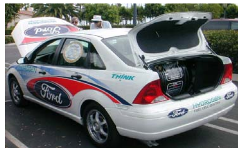
Ford Hydrogen Fuel Cell Vehicle (FCV): The hydrogen tank (at 5000 psi) is stored inside the trunk (above). Under the hood with the fuel cell engine (below).
