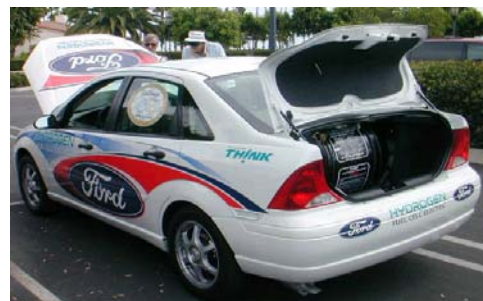
Ford Hydrogen Fuel Cell Vehicle (FCV): The hydrogen tank (at 5000 psi) is stored inside the trunk (above). Under the hood with the fuel cell engine (below).
